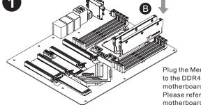
Plug the Memory Module(B) to the DDR4 slot on the motherboard.
